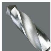
Twist drill bits - for metal applications • ¼" drive suitable for holders as per DIN 3126-D 6.3 (ISO 1173) • Hexagon shaft for very high torque transfer • HSS = high speed steel with cone point • Finely adjusted material elasticity for long service life • Excellent concentricity • Tough-absorbing tempered bits for particularly long service life
